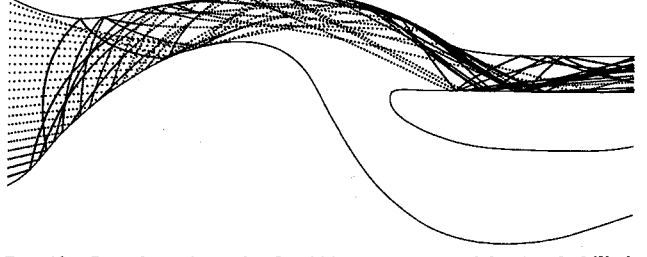
Fig. 10 Sample trajectories for 200- \mu m sand particles (probabilistic bounce model).
